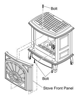
Figure 41 - Removing Front Panel from Stove
